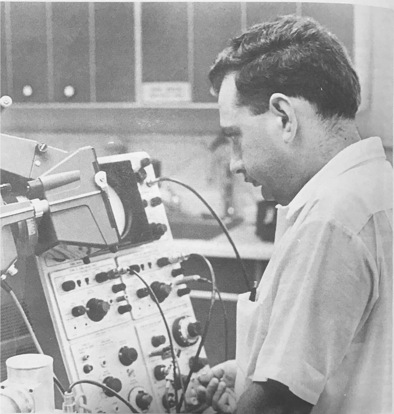
Dr. Jacob Levinson, of Israel, detecting radiation damage in anthracene crystals by using non-linear optical methods with a cathode ray oscilloscope and a 100 mw Q switch laser
