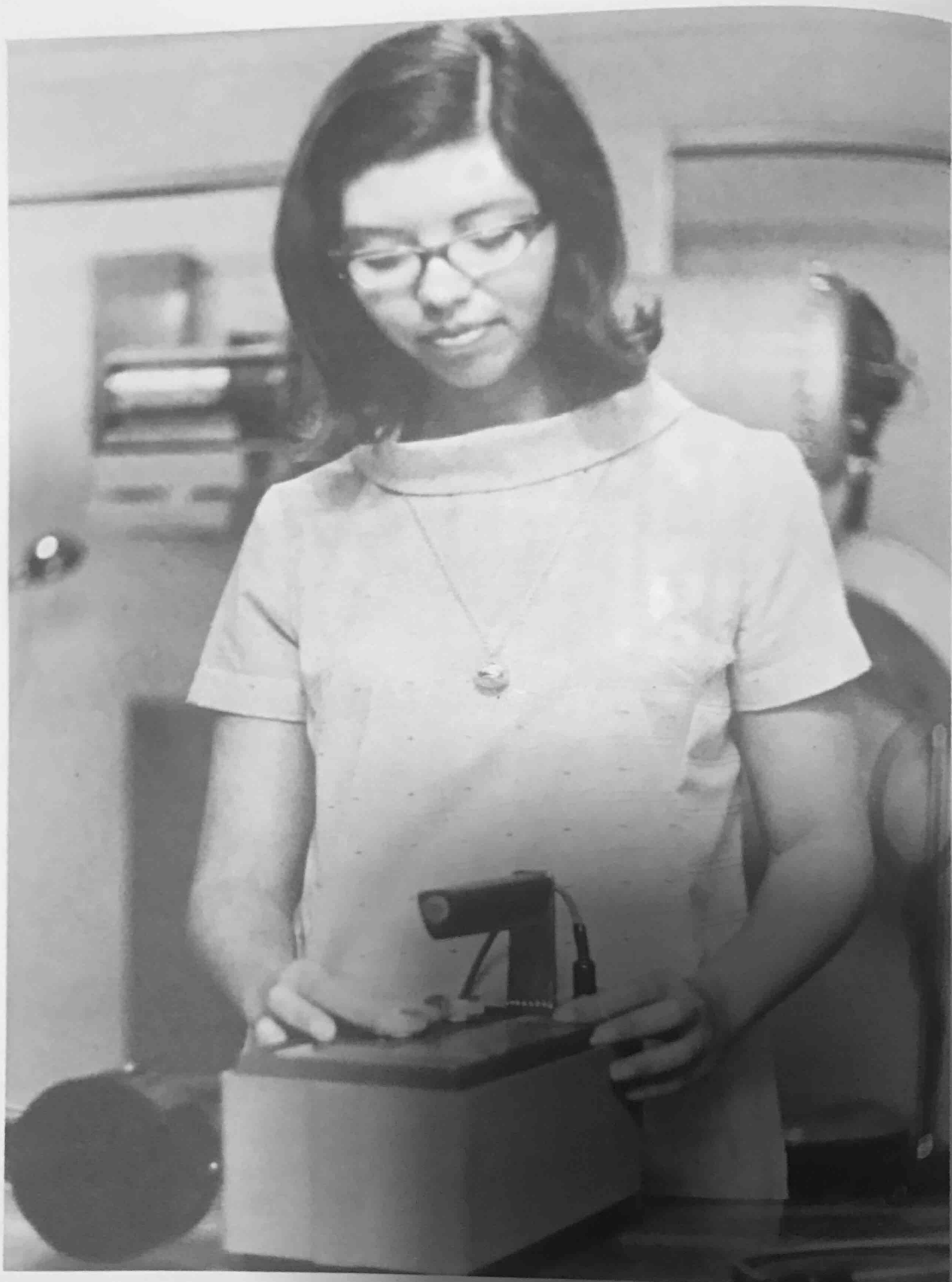
Miss Heidi Pabón Pérez sets up x-ray detection equipment used with diagnostic and therapy x-ray units to measure direct beam and stray radiation
