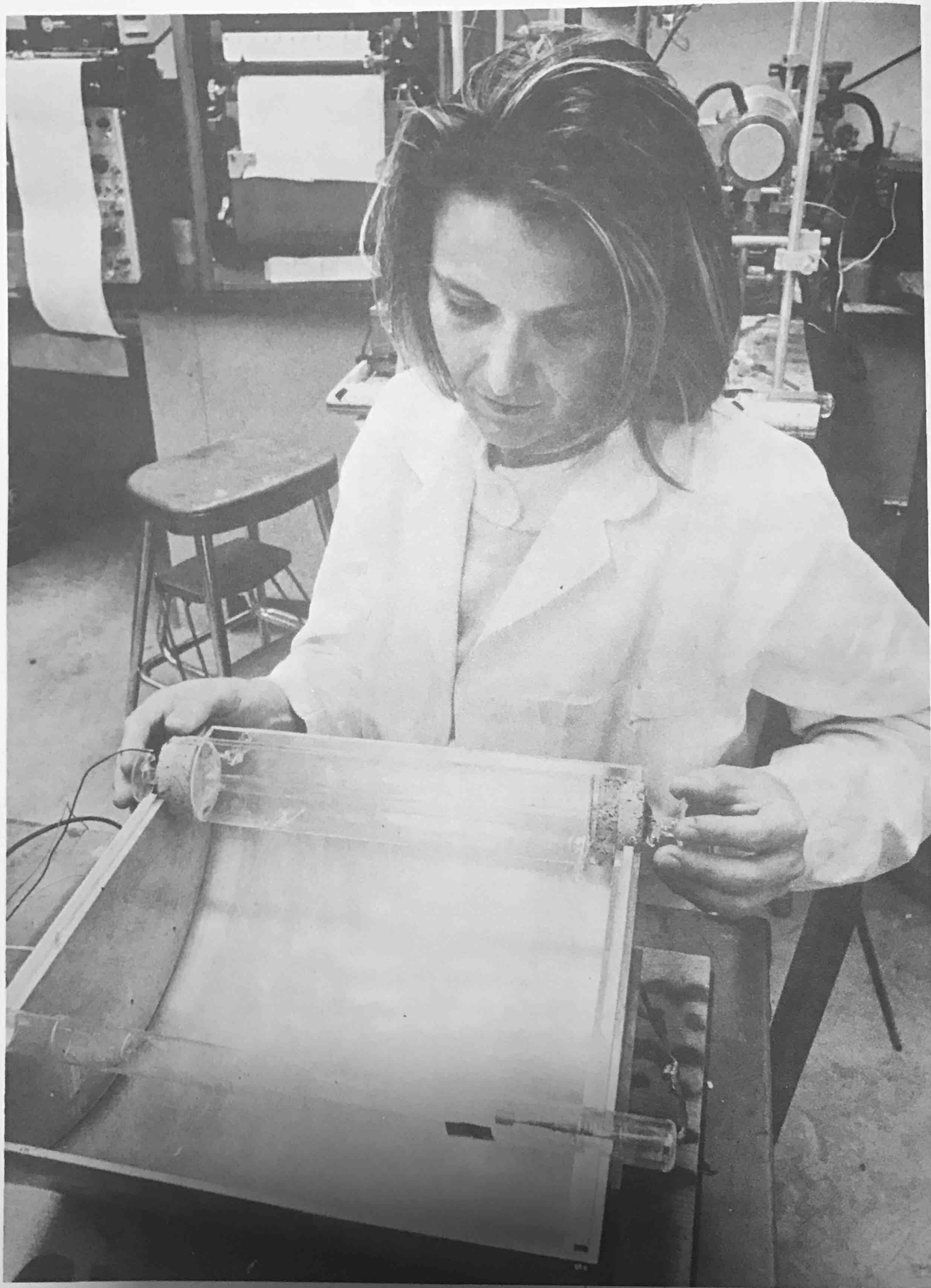
Mirtha Trujillo Sánchez, a Cuban chemistry graduate student, examines the flash photolysis apparatus
