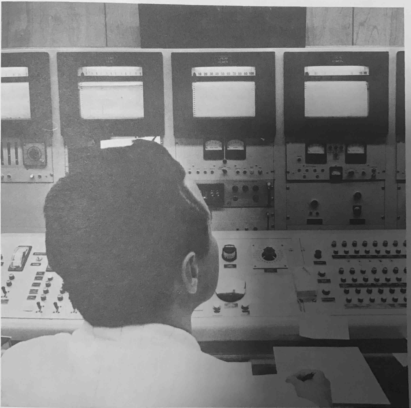
Operator observes the one megawatt reactor console and instrumentation rack
