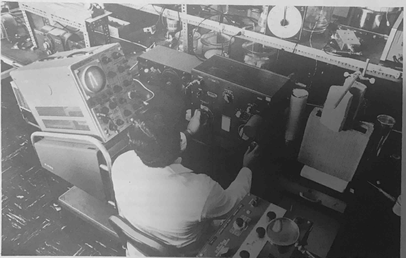
Ivan Nazario does temperature dependent capacitance measurements using the following equipment: R.F. oscillator, capacitance bridge, potentiometer, and oscilloscope
