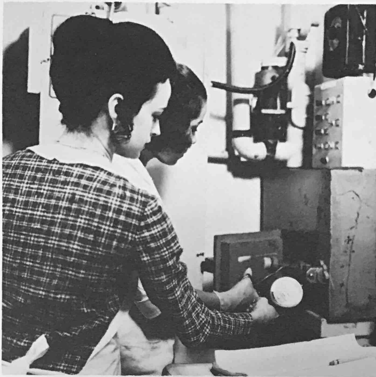
“Rabbit” being removed from receiver for neutron activation analysis for trace elements.
