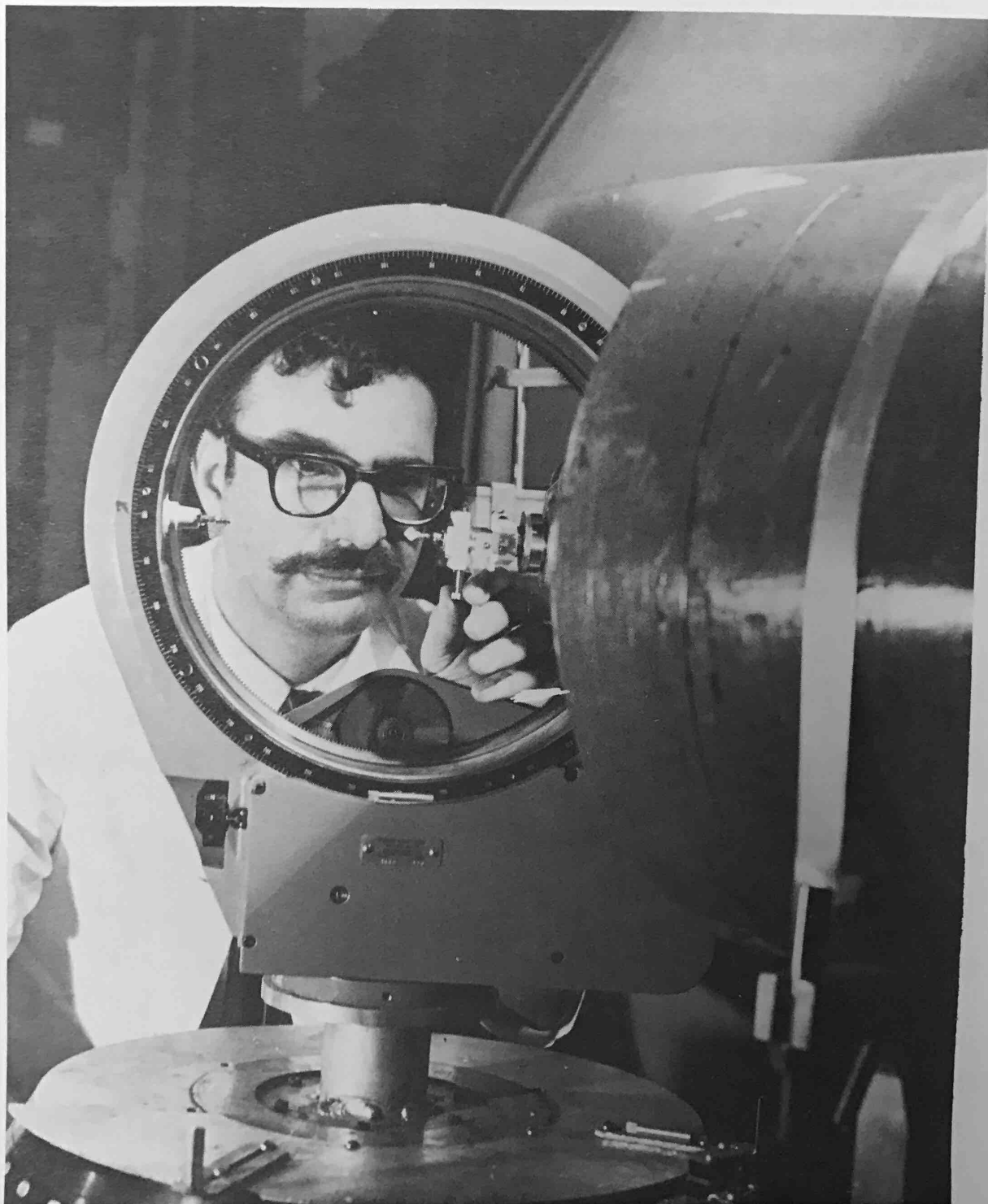
Dr. Mortimer Kay mounting crystal on circular goniometer for neutron diffraction studies.
