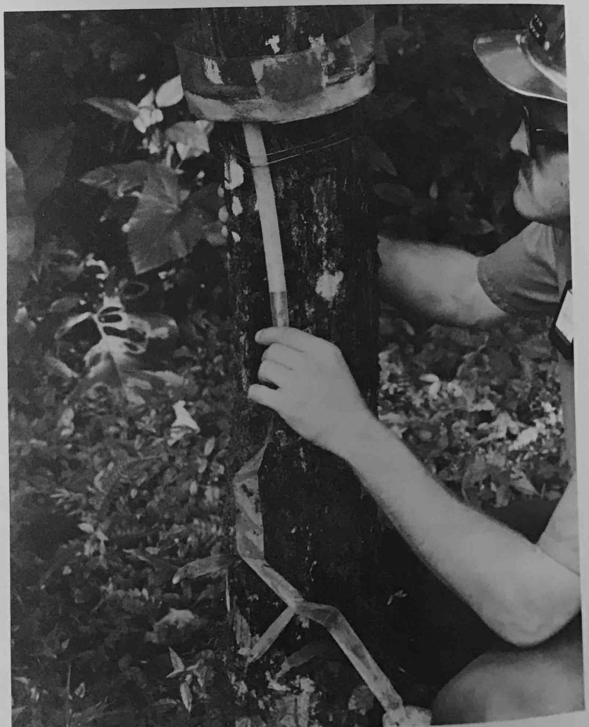
W. C. Dirk reviewing installation of a stemflow collar used in Rainfall-Interception studies at El Verde.
