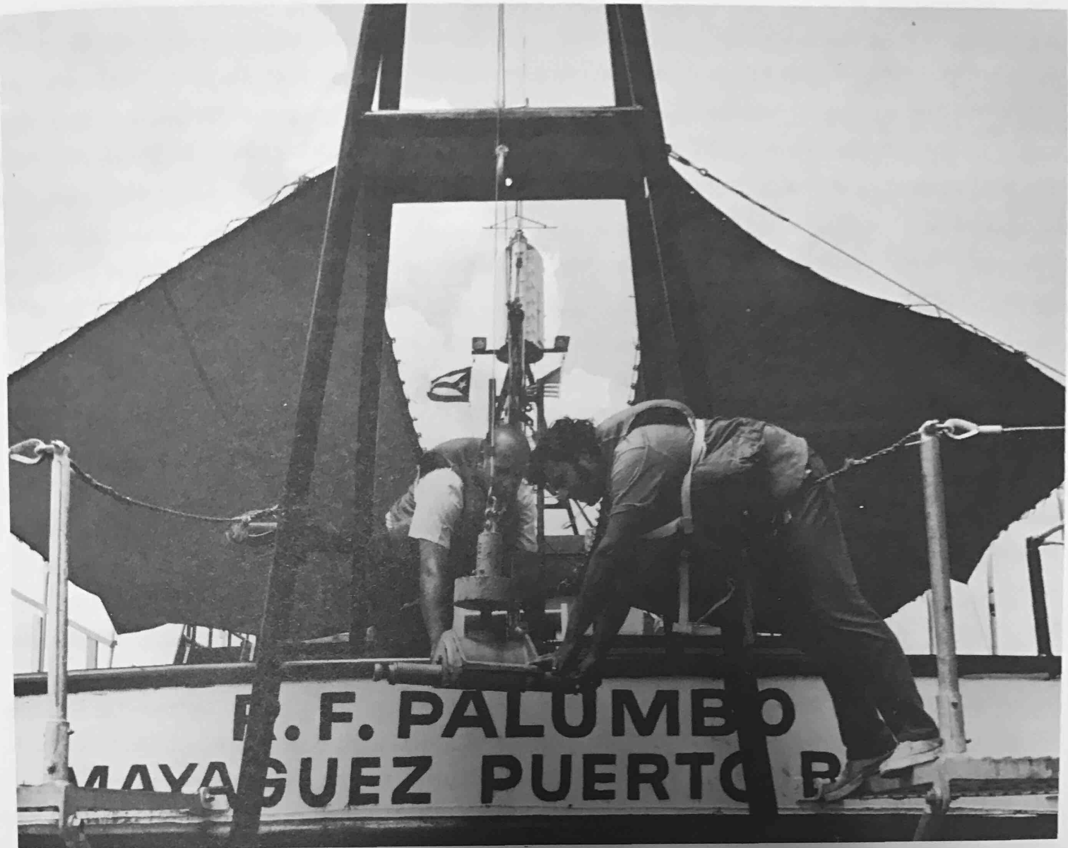
Mr. David Brunet, Engineer, and Mr. Edwin Jusino, Mate, in charge of sampling gear aboard the research vessel R. F. Palumbo working with Shipek bottom grab in Mona Pass. Bottom samples are later prepared for trace element analyses.
