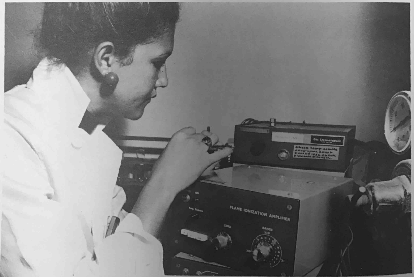
Miss Carmen Vega, working with gas-liquid chromatography to separate silyl derivatives of ^{14}\text{C} -labeled amino acids.
