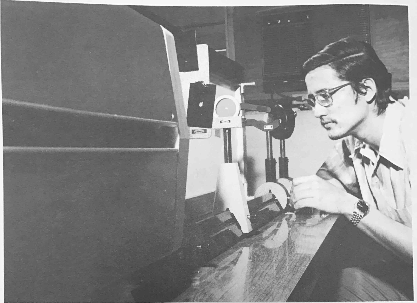
Mr. Aurelio Mercado, graduate student in Physics, using laser beam for Brillouin scattering studies.
