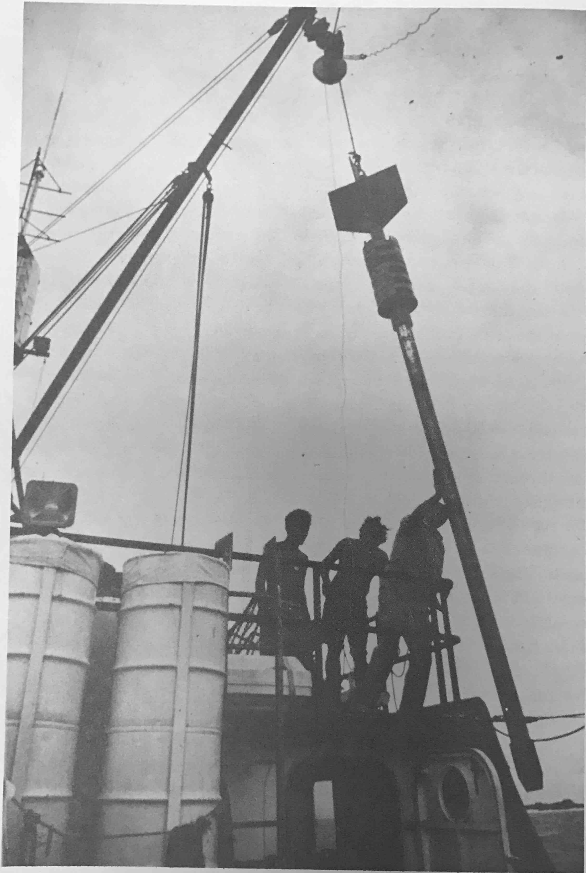
Operation of a large corer on the Palumbo in the Bravo bomb crater on Bikini Atoll. The large white tanks on the left were used to coprecipitate transuranium elements in seawater samples.
