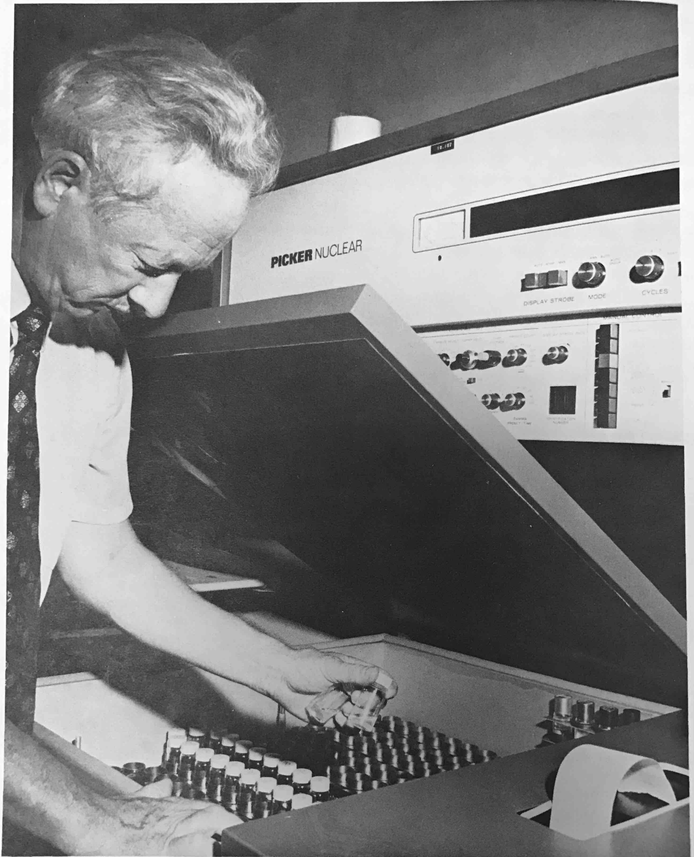
Dr. Raymond A. Brown using the scintillation counter to measure binding of ^{131}\text{I} -labeled S. mansoni antigen.
