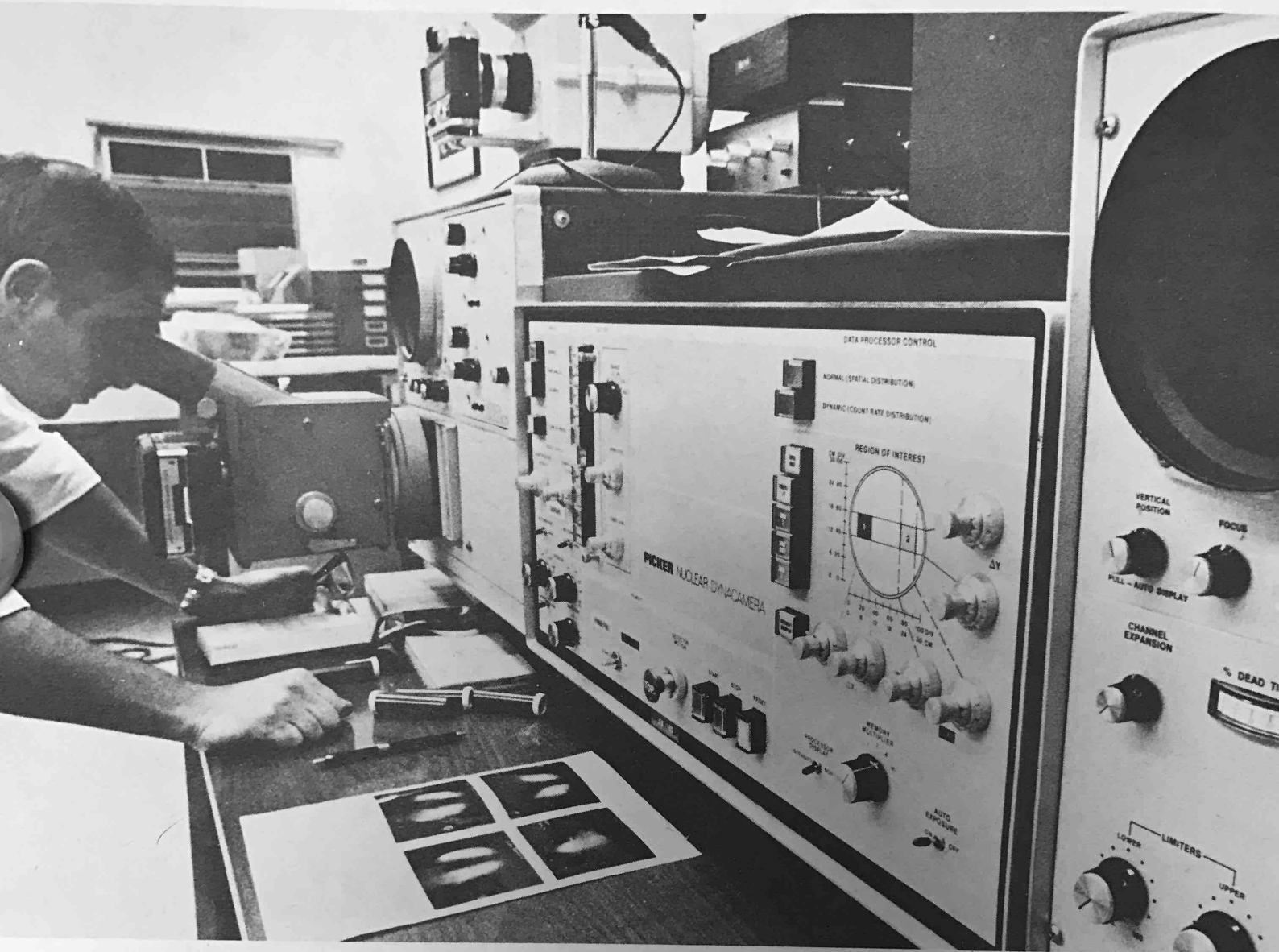
A view of the Anger Camera Console showing the complex controls needed for the operation of this versatile equipment.
