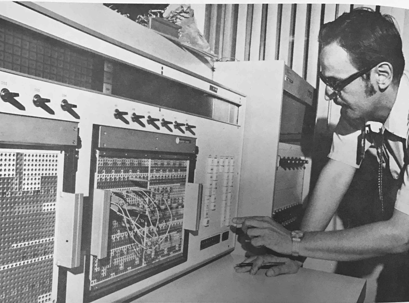
Dr. Arthur McB. Block checking variable resistance circuits and operational amplifiers of a Comcor 175 analogue computer acquired recently by the Terrestrial Ecology Division from U.S. Government surplus. The analogue computer may aid in the interpretation of environmental data obtained in the Espiritu Santo watershed.
