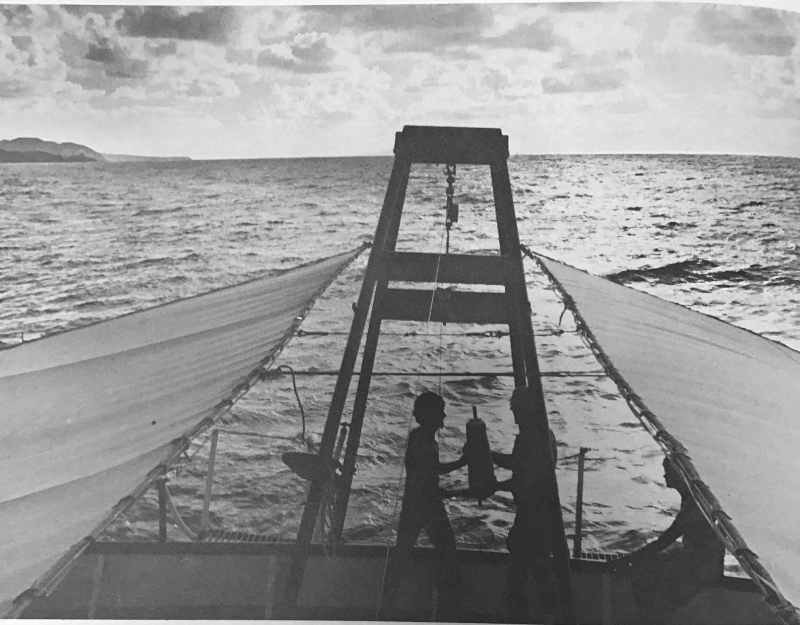
The A-frame and winch apparatus aboard the R. F. Palumbo used in marine ecology studies. E. D. Wood, assisted by technicians, readies a water sampling bottle which will be lowered into the sea off the west coast of Puerto Rico
