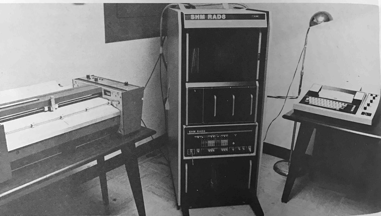
This SHM Rad 8 Radiotherapy treatment-planning system was installed in the Radiation Oncology division in May 1975. At right is the control keyboard and tablet for feeding patient contour into the computer. In the Center is the Assembly of PDP-8 computer, the memory disc drive unit and storage oscilloscope display unit. At the left is the plotter for producing a copy of the completed treatment plan.
